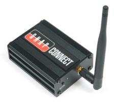
The *SNAP Connect* E10 is basically a small Linux computer that comes with *SNAP Connect* preloaded.
