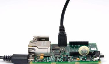
**Step 3:** Remove jumper J5. You may need needle-nose pliers to remove the jumper that resides directly behind the LED mounting next to the SNAP Engine on the "wireless" end of the E10. You might find it helpful to remove the SNAP Engine first for easier access to the jumper, as shown in this picture.
