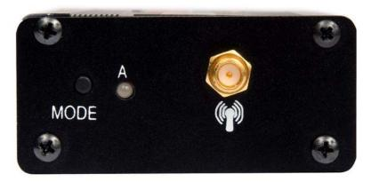
As delivered, LED A glows green when the E10 is powered. Holding the Mode button during startup causes the E10 to bypass the standard SNAP Connect software in the unit. Holding the Mode button for 10 seconds causes the E10 to perform an orderly shutdown.
