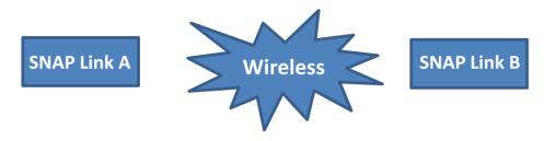
Under certain conditions it may be necessary to extend the range between two SNAP links. This could be conditions related to interior walls, equipment, doors, anything that can impede the RF signal. In cases like this you may be able to re-establish the wireless link with a SNAP link configured as a repeater.
